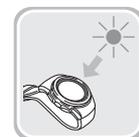
While you are wearing the watch, make sure that its face (solar panel) is not blocked from light by the sleeve of your clothing. Power generation efficiency is reduced even when the face of the watch is blocked only partially.
